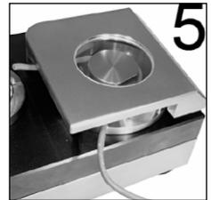
6. When you open the protection cover, the pull force fixture returns back to the original position and releases the cable.
